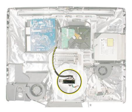
Using a torx T10 screwdriver, remove the three 7-5-mm long self-tapping screws from the power inlet and the 5-mm long machine screw from the ground cable . Remove any EMI tape on the metal case.
